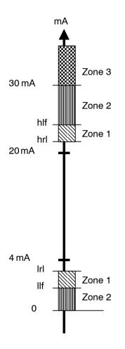
When the measured value is in Zone 1, the default action is to approve the newest measurement read from the I/O unit and add the fault bit 'OVF' to it. The Zone 1 limits are specified using the configuration symbol parameters "Measurement low limit" (lrl), "Line fault low limit" (llf), "Measurement high limit" (hrl) and "Line fault high limit" (hlf). Measurement processing and the operation of the OVF fault bit can be controlled with the "Line fault control" (lfcntrl) parameter.
